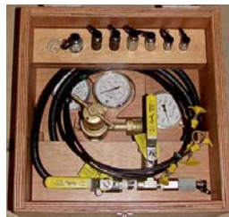
BLEEDING VALVES AND CHARGING KITS ALLOWS CONTROLLED BLEEDING AND FILLING UP OF IZERWAREN GAS SPRINGS. See page 6-13 page
